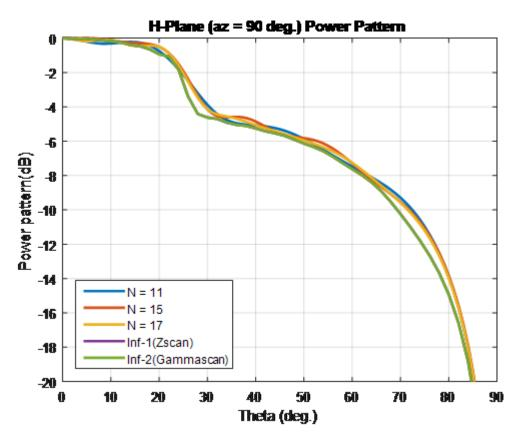
For finite arrays of size greater than  $10 \ge 10$ , the scan element patterns in the E-, D-, and H-planes match the patterns of the infinite array scan element.
