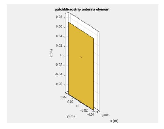
The patch lies behind the ground plane and is not visible. To make the patch visible (in front of the ground plane), rotate the antenna about the negative y-axis.
