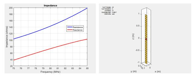
In above example, the dipole is meshed at the highest frequency, 85 MHz automatically before calculating the impedance at all the frequencies from 75 to 85 MHz. Meshing at the highest frequency, 85 MHz, ensures maximum number of triangles and a smoother plot of the dipole impedance. Use the mesh command to view the meshed dipole. The number of triangles is 48, which is more than single frequency meshing.
