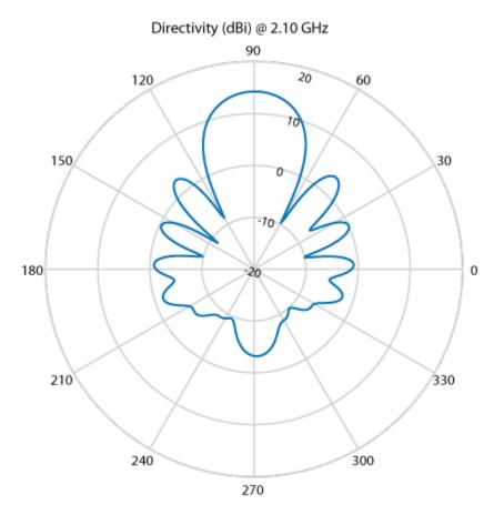
*Half power beamwidth* (HPBW) is the angular separation in which the magnitude of the radiation pattern decreases by 50% (or -3dB) from the peak of the main beam
