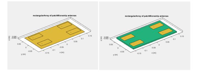
For example, the voltage vector matrix for a 2x2 array of rectangular patch antenna (with and without dielectric substrate) has four columns as each antenna can be excited separately.
