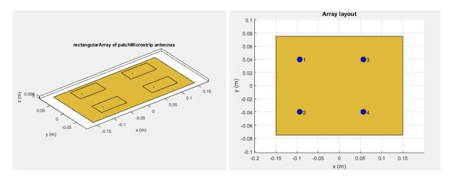
For example, the voltage vector matrix for a 2x2 array of rectangular patch antenna has four columns as each antenna can be excited separately.
