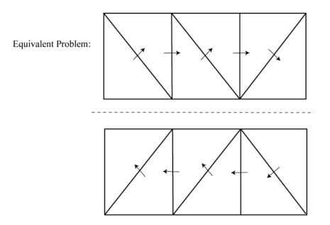
According to the method of images, the real and image electric currents are equal to each other in terms of magnitude. The parallel components are in opposite direction. The normal components are in the same direction.
