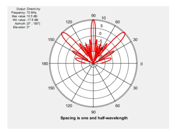
The grating lobes move in or out of the visible region depending on the spacing between the elements and the relative phase between them.
