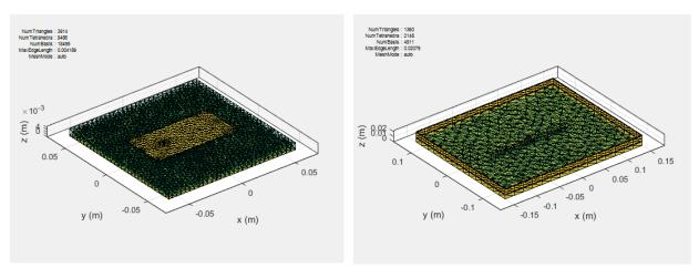
the metal surface of the antenna is meshed into triangles and the dielectric volume is meshed into tetrahedrons.
