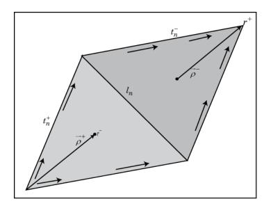
The basis function includes a pair of adjacent (not necessarily coplanar) triangles and resembles a small spatial dipole with linear current distribution. Each triangle is associated with a positive or negative charge.
