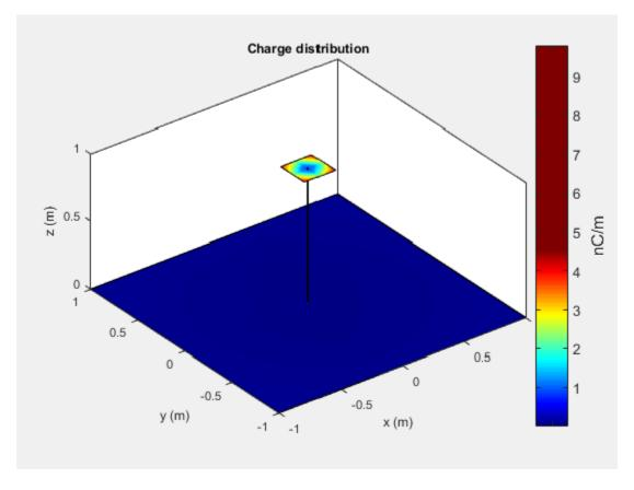
The increase in capacitance lowers the frequency of the antenna. By keeping the physical volume of the antenna same, the resonance point is shifted.
