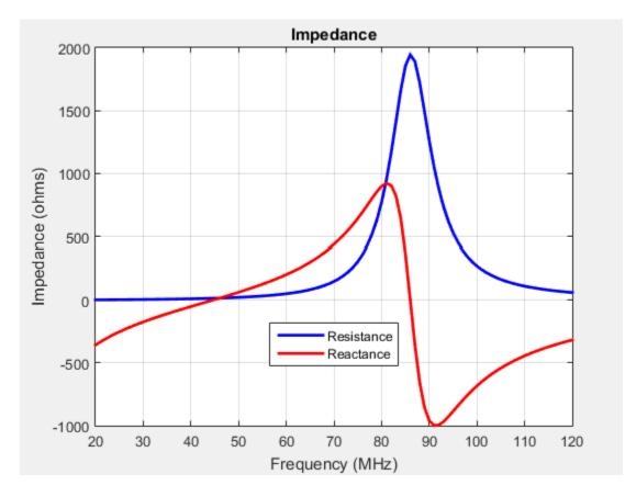
All the dimensions of this antenna are same as the monopole. The first resonance of the antenna is approximately 45 MHz. To view the accumulated charges on the top-hat monopole, use the **charge** function:
