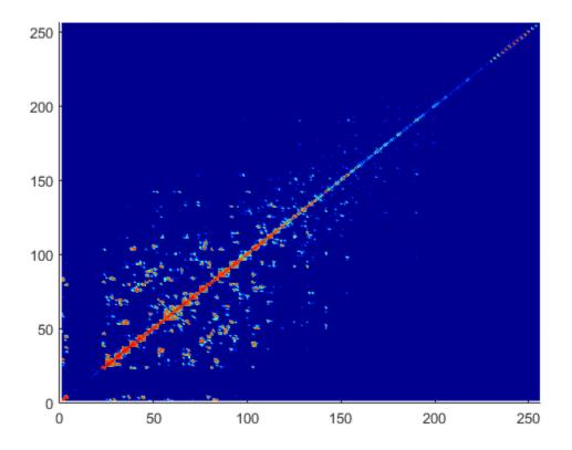
To fill out the interaction matrix, calculate the free-space Green's function between all basis functions on the antenna surface. The final interaction matrix equations are:
