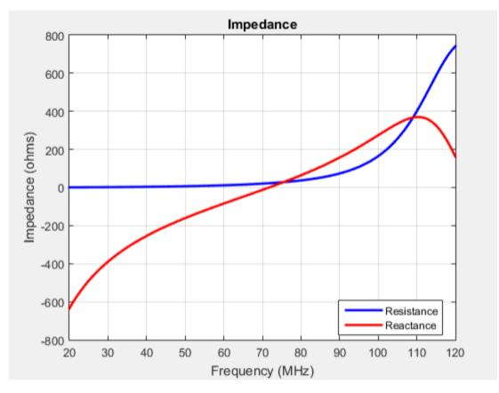
You can observe the first resonance is at approximately 71 MHz. To lower the resonance frequency, recalculate the height of the monopole to quarter wavelength. The frequency of operation is also lower. You must also have to increase the size of the corresponding ground plane. This increase in size means that to achieve similar performance at a lower frequency, you need a larger antenna. This approach is not possible due to physical space constraints.
