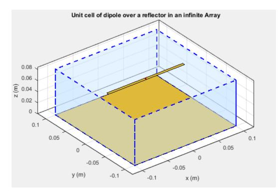
The dotted blue box bounds the unit cell. Ground plane length and ground plane width of the unit cell are the dimensions of the antenna element of the infinite array.
